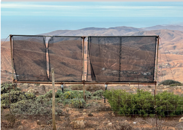
Fig. 8 Fog harvesting nets for water collection on Fuerteventura (Photo: Laura Dierksmeier).
